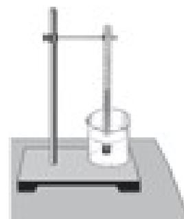
Observe till the mercury thread in the capillary tube becomes steady and read the level of mercury. This reading gives the temperature of tap water taken in the beaker.
